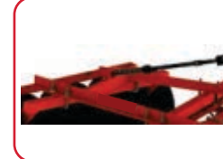
Gang adjustment on U clamp
