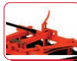
Gang angle adjustable on handle.
