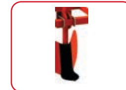
Tyne can adjust easily with help of clamp
